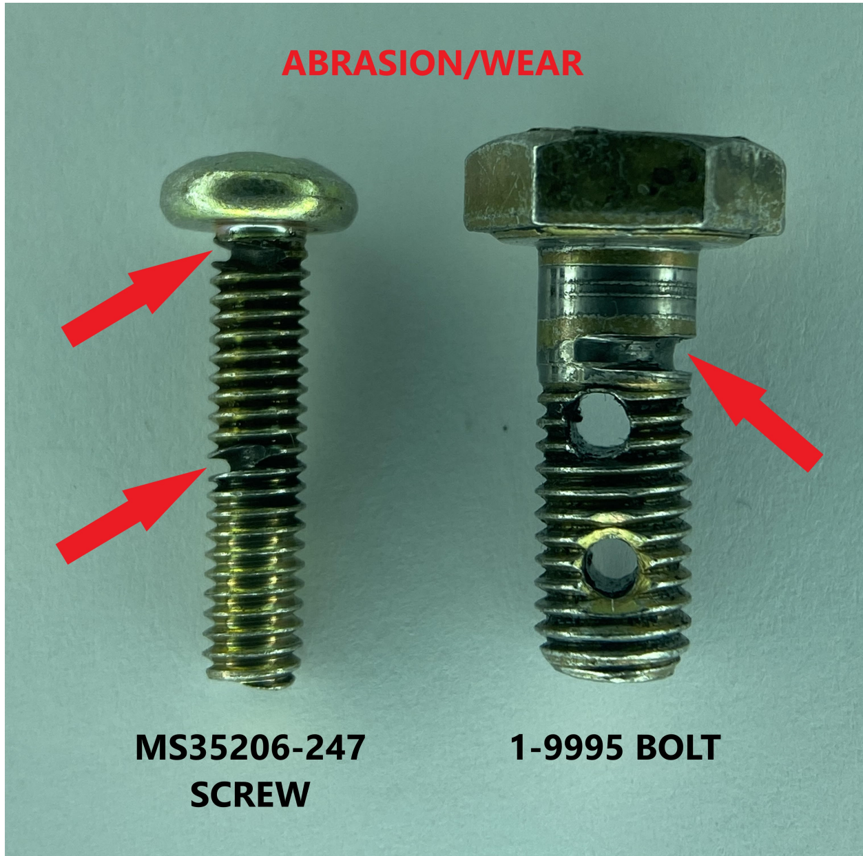
Figure 1: Example of Abrasion/Wear of Air Box Hardware
